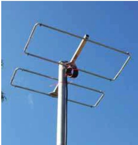
PHOTO 2: The 2m version of the Super Moxon is just 30" x 25".
